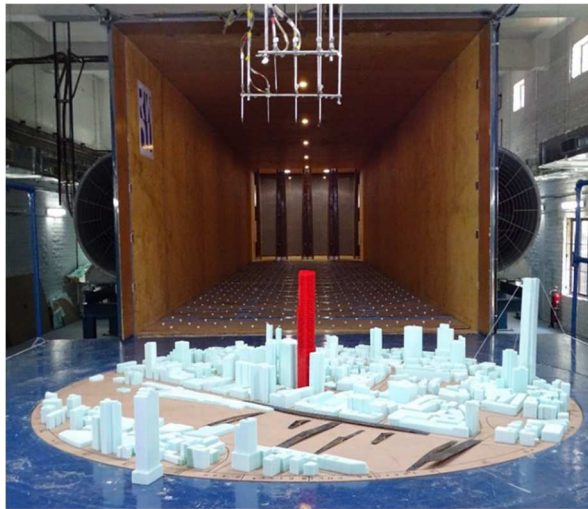
Figure 5. Wind Tunnel Study Model
